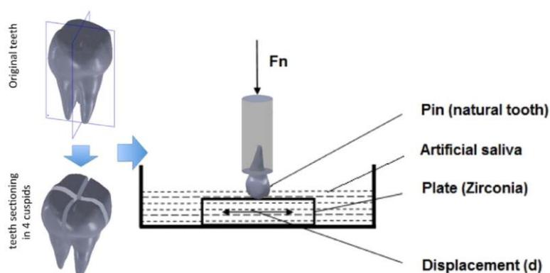
**Figure 2.23:** Schematic representation of the reciprocating wear test (Buciumeanu *et al.*, 2017).
