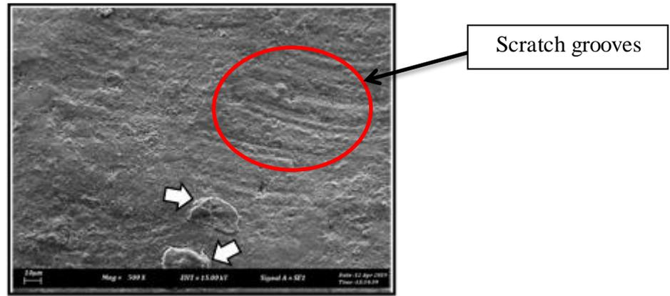
**Figure 2.12:** SEM image with scratch grooves of specimen (x500). Micro-pitting is shown in the arrow (Hamid *et al.*, 2019).
