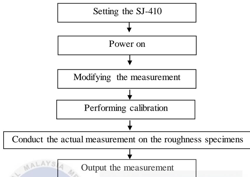
**Figure 3.14:** The measurement flow for surface roughness test.
