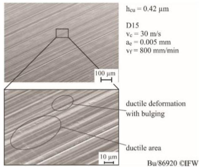
**Figure 2.19:** Surface topography of ground surface with  $h_{cu} = 0.42 \mu\text{m}$  (Denkena *et al.*, 2017).
