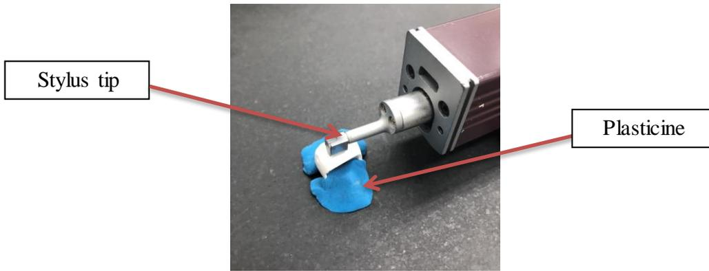
**Figure 4.2:** Sample setup with plasticine support.
