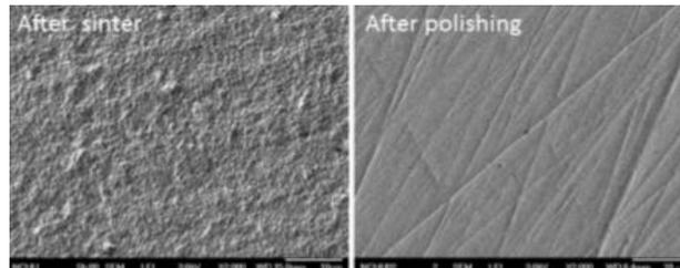
**Figure 2.14:** SEM photomicrographs with 2000x magnifications of blasted Zirconia surfaces showing surface morphology after sintering and after polishing process (Cheng *et al.*, 2018).
