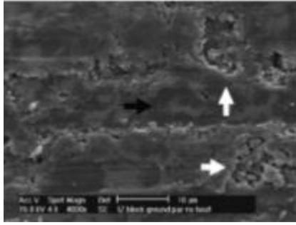
**Figure 2.17:** SEM images with 4000x magnification without heat treatment. The black arrow indicates the direction of grinding; the white arrows indicate major defects whose shape and orientation seem unrelated to the grinding orientation (Guazzato *et al.*, 2004).
