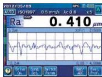
Figure 3.16: Example of measurement on Mitutoyo Surftest SJ-410.
