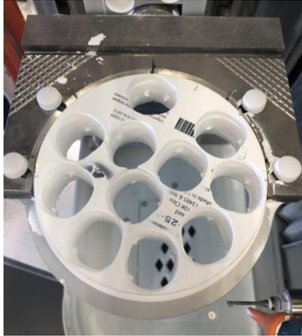
**Figure 3.10:** Zirconia block after machining.
