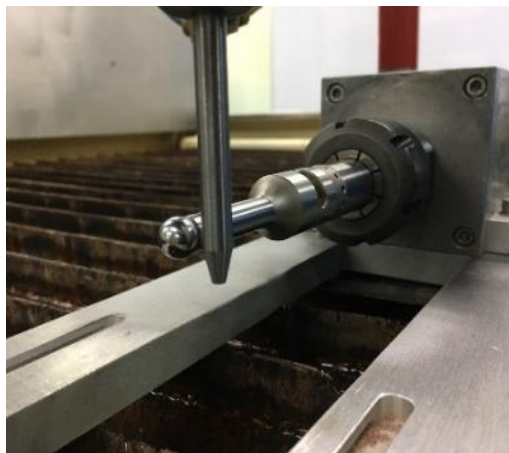
Figure 3.10: Zero position of Y-axis by using an electronic edge finder
