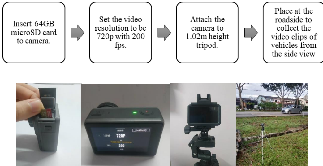
Figure 3. 4: Procedure for setup of camera.
