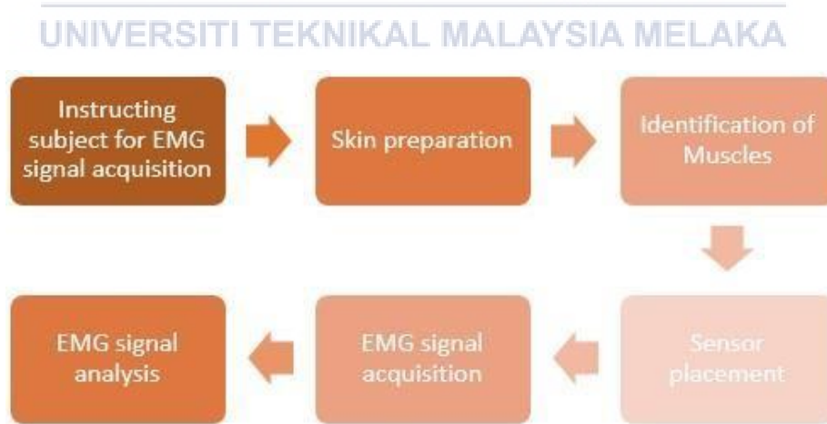
Figure 3.7: Steps of electromyography testing of GA patient. ( EMG manual, 2017)
