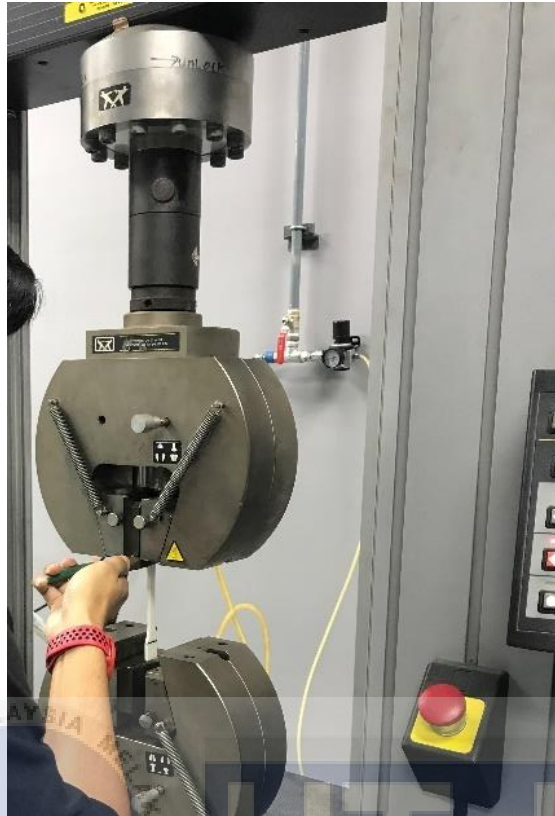
Figure 3.13: Process of placing the specimen
