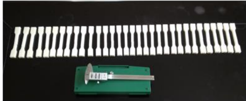
Figure 2.6: Thirty-two dogbone ABS specimens for tensile test
