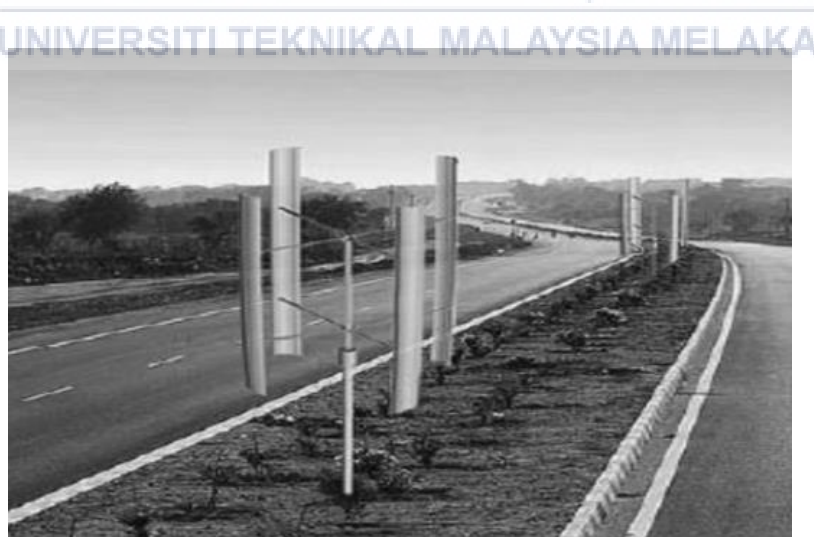
Figure 1.1: Example of Vertical Axis Wind Turbine that Installed in highway
