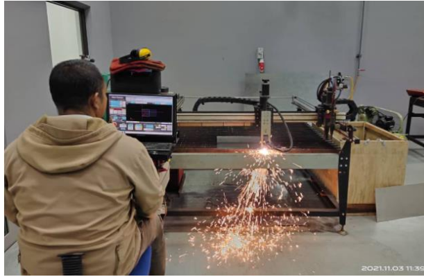
Figure 3.18: Process of Cutting Material using CNC Plasma Machine
