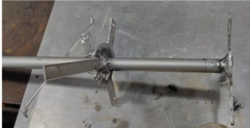
Figure 3.20: Defects that Happened During Using TIG Welding as Joiner
