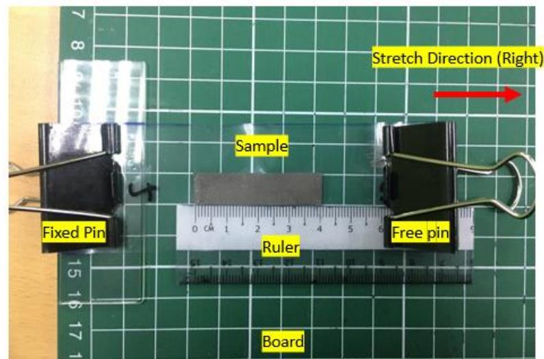
Figure 3.13: Manual Cyclic Stretch Test Setup
