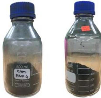
Figure 3.2: Graphene Nanoplatelets (GNP) of 5 $\mu$ m and 15 $\mu$ m
