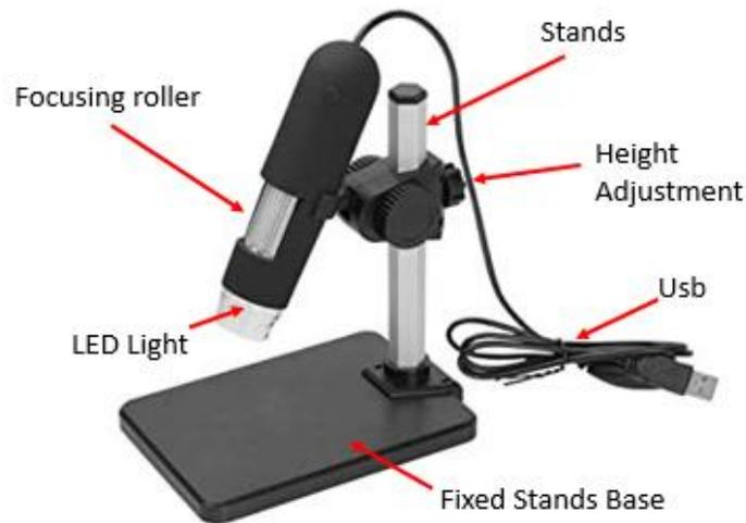
Figure 3.19: Digital Microscope
