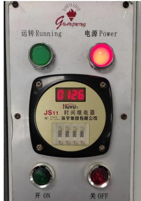
**Figure 3.6:** Pulveriser machine (set at 500 seconds per process)
