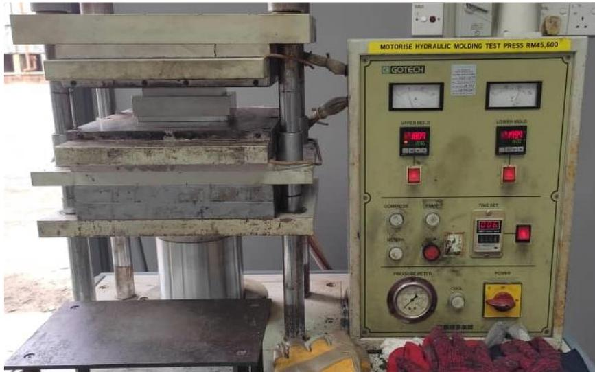
**Figure 3.8:** Hydraulic hot press machine
