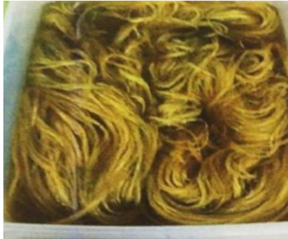
**Figure 3.4:** Kenaf fiber soaked in NaOH solution
