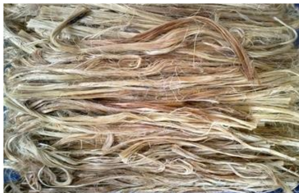
Figure 2.1: Kenaf fiber before treatment
