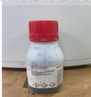
Figure 3.2 Sigma Aldrich PEDOT: PSS with 1.3 wt. % dispersion in the \text{H}_2\text{O} polymer binder
