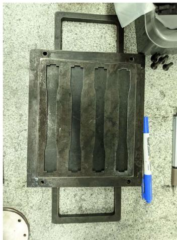
Figure 3-9: Mould for bone shape.
