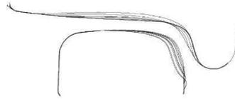
Figure 2-4: Form change of wheel and rail over a two-year period from the Stockholm test case. (Roger Lewis & Olofsson, 2009)
