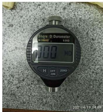
Figure 3-13: Shore Hardness Durometer-D.
