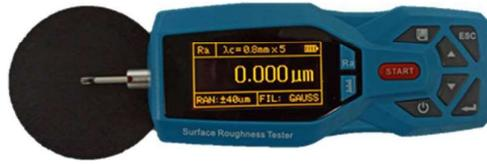
Figure 3-14: Surface roughness tester profilometer.
