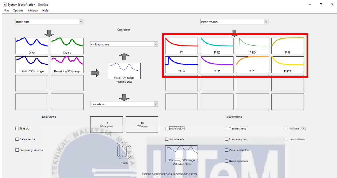
Figure 3.16: Displayed estimated process models based on working data
