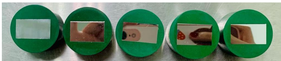
Figure 3.5: Surface of samples after polishing.
