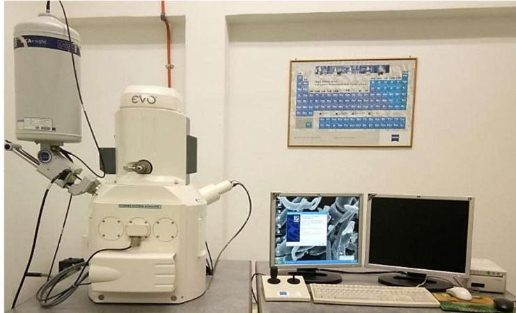
Figure 3.9: Scanning Electron Microscope (SEM) for fracture surface morphological observation
