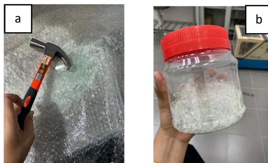
Figure 3.3: (a) The hammering using claw hammer (b) The final size of manual crushing
