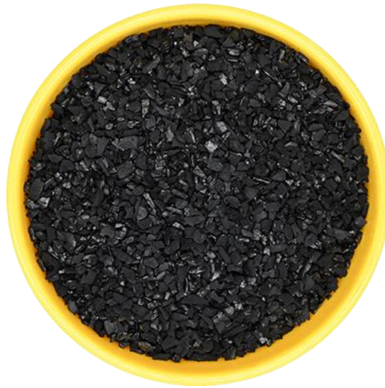
Figure 2.4: Granular Activated Carbon (GAC) (khy, 2021)
