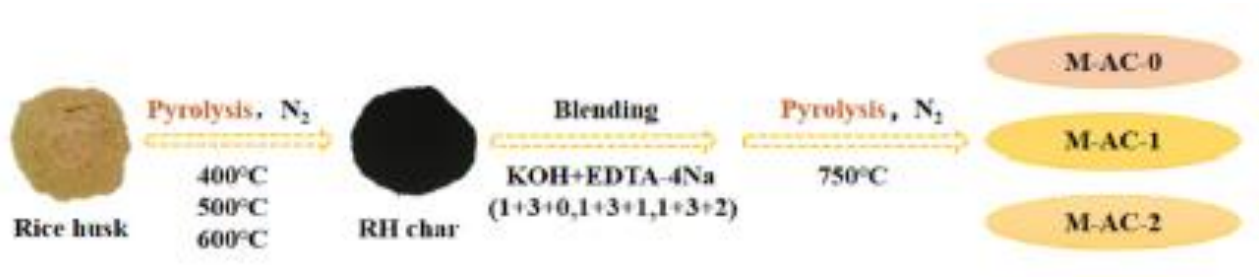
Figure 2.9: Rice husk pyrolysis diagram and alteration of activated carbon (Lv et al., 2020)
