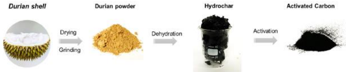
Figure 2.11: Schematic diagram of preparation activated carbon via acidis dehydration of durian husk (Ukkakimapan et al., 2020).
