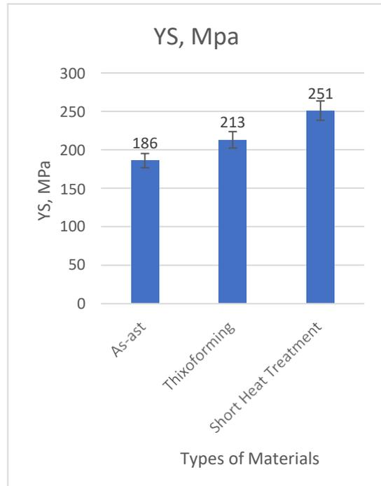
Figure 4.8: Graph of Tensile Test Result for A319 – MWCNTs Composite Alloy; a)UTS and b) YS
