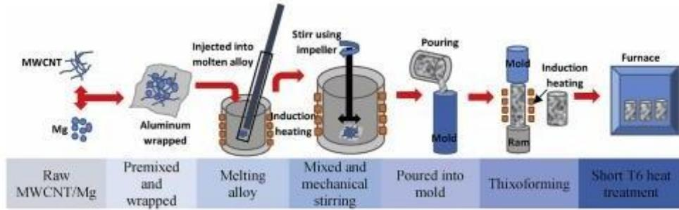
Figure 2.10: Mixing Process involved Short T6 Heat Treatments ( Salleh et al., 2019)
