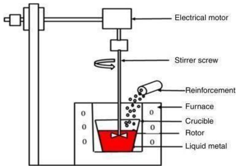
Figure 2.5: Stir Casting Method (Thandalam et al., 2015).
