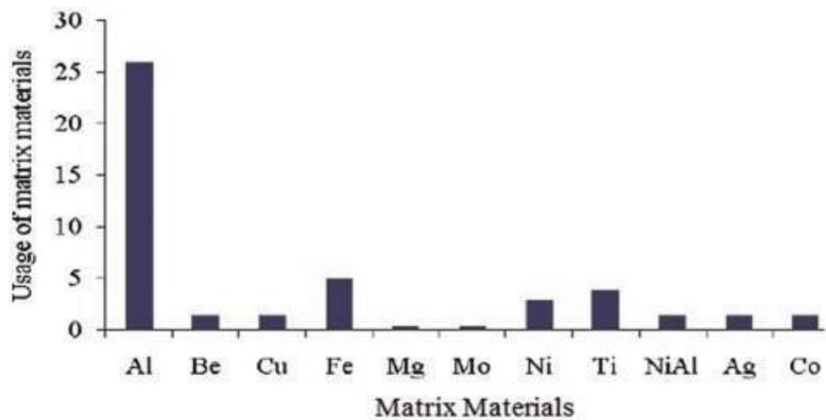
Figure 2.3: Usage of matrix material in MMCs (Adebisi et al. 2011).
