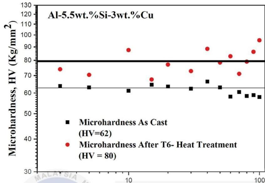
Figure 2.25: Microhardness after as- cast and after T6 Heat Treatment (Magno et al., 2017).
