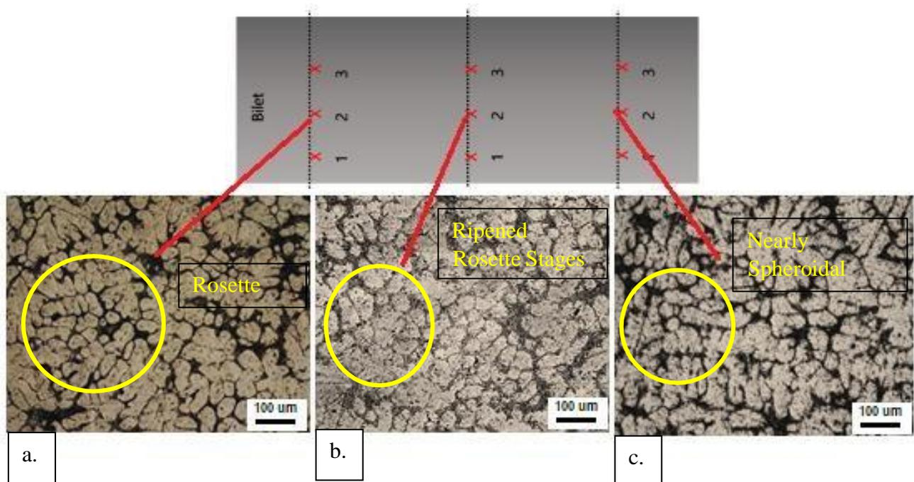
Figure 4.2: Microstructure Of Feedstock Material After Cooling Slope Process
