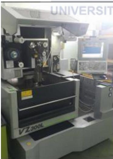
Figure 3.13: Wire Cut EDM Machine from FKP Laboratory
