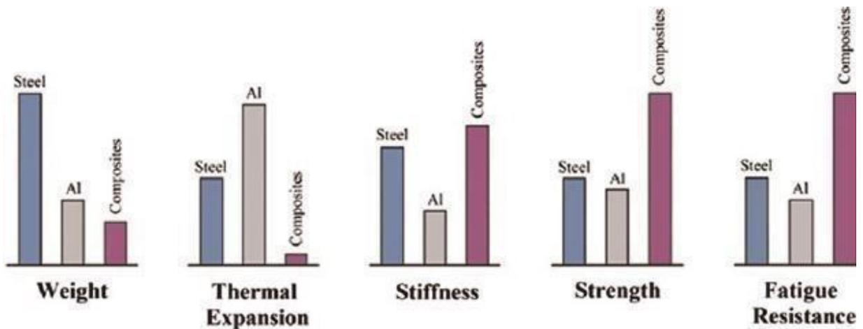
Figure 2.2 Properties of composite as compared to most commonly used alloys, steel and aluminium.
