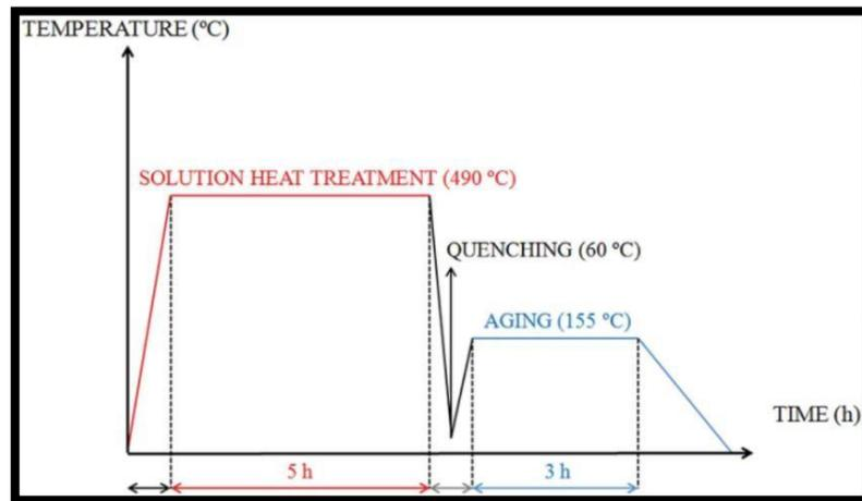
Figure 2.9: Stages of T6 heat treatment applied represented schematically (Magno et al., 2017).
