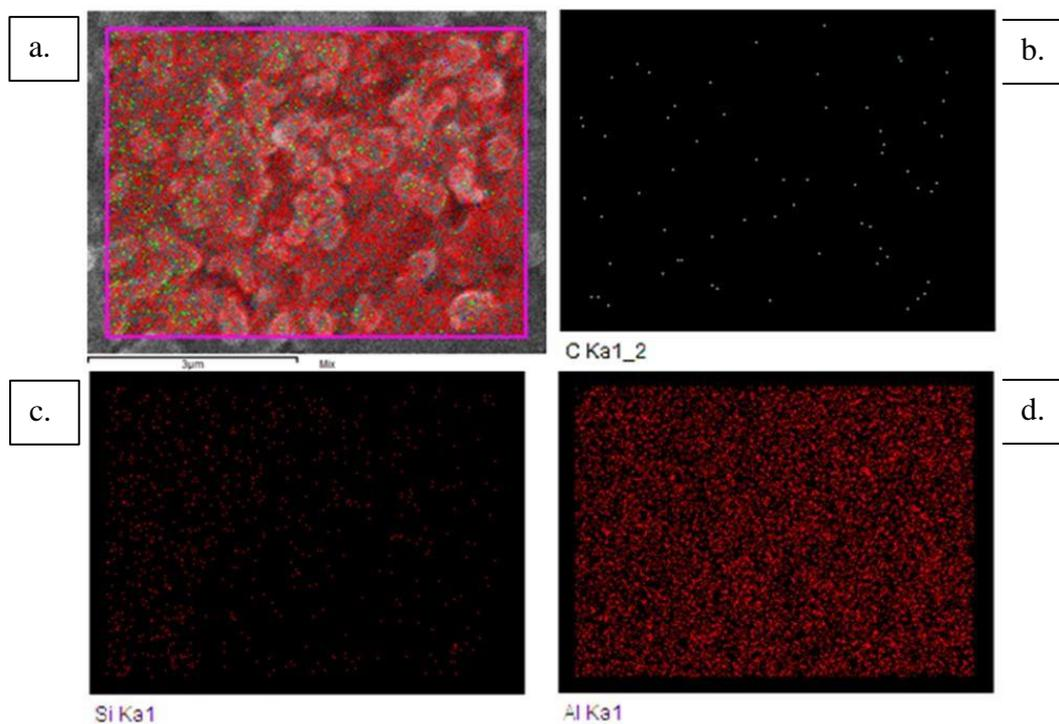
Figure 4.5: SEM – EDS Analysis of MWCNTs – A319 Composite Alloy
