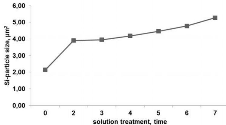
Figure 2.26: Graph of the effect of solution treatment in times on Si particle size (Tillová et al., 2018).
