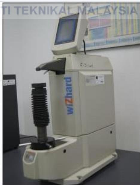
Figure 3.10: Rockwell Hardness Tester
