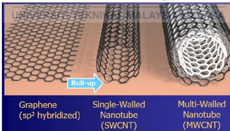
Figure 2.13: Schematic Diagram How Cnts Can Be Produce By Graphene Ideally (Hammond Et Al., 2016).
