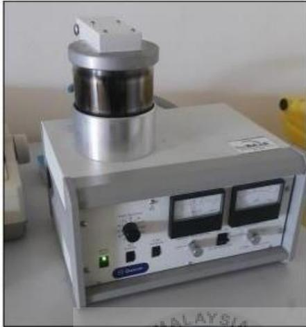
Figure 3.17: Mini Sputter Coater from FKP Laboratory
