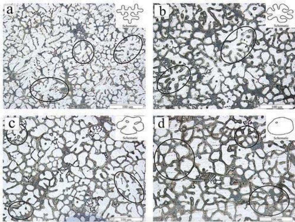
Figure 2.21: (a) impact zone, (b) top zone, (c) middle zone and (d) bottom zone for microstructure of A319 (Aziz et al., 2016)
