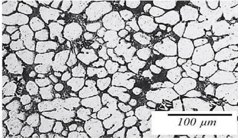
Figure 2.22: Microstructure of A319 aluminium alloy after CS casting process (Salleh, 2014).
