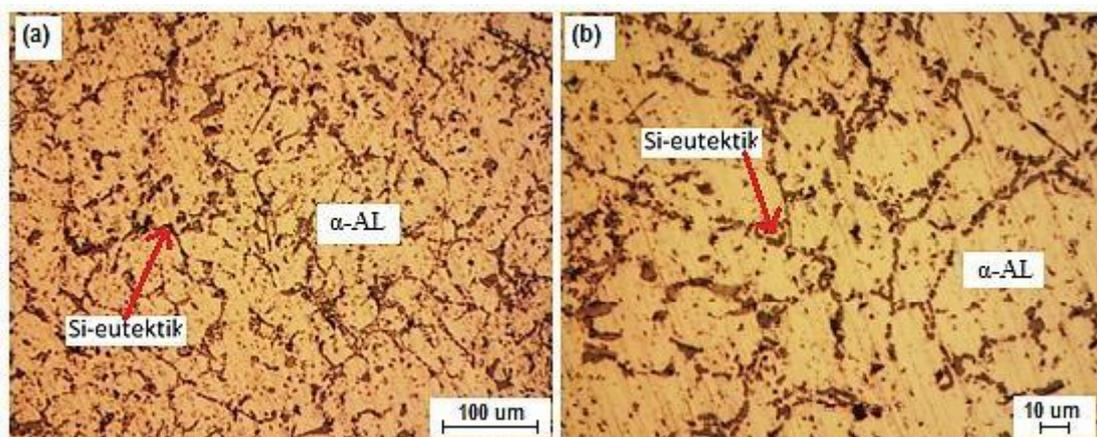
Figure 4.3: Microstructure after thixoforming of A319- CNTs Composite Alloy
