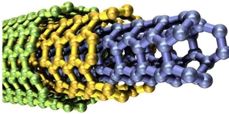
Figure 2.17: Schematic illustration of MWCNTs (Aman et al., 2015).
