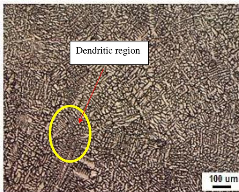
Figure 4.1: Microstructure of Raw material A319
