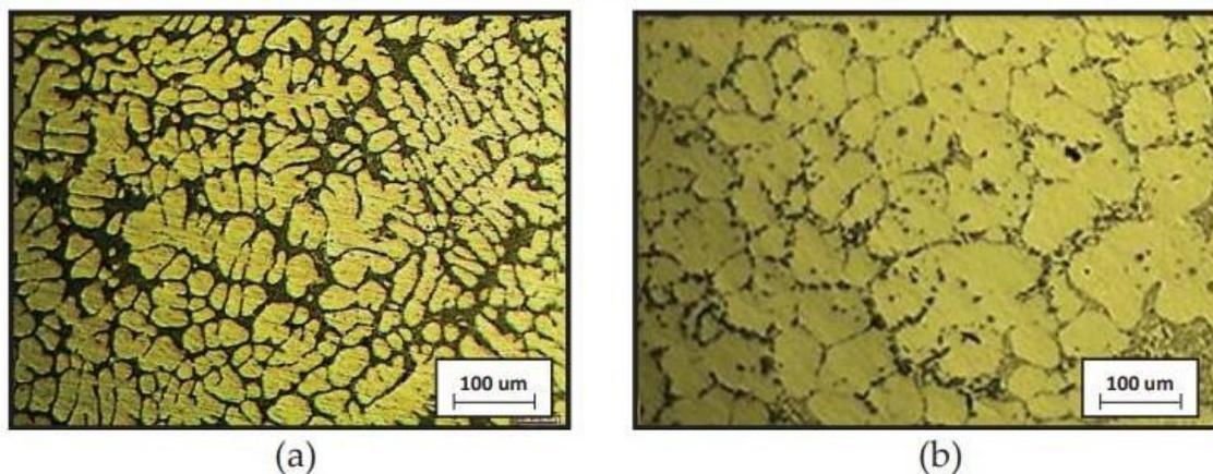
Figure 2.24: Microstructure of (a) as-cast of A319 aluminium alloy and (b) Thixoformed A319- MWCNTs Composite Alloy (rahman et al., 2020).
