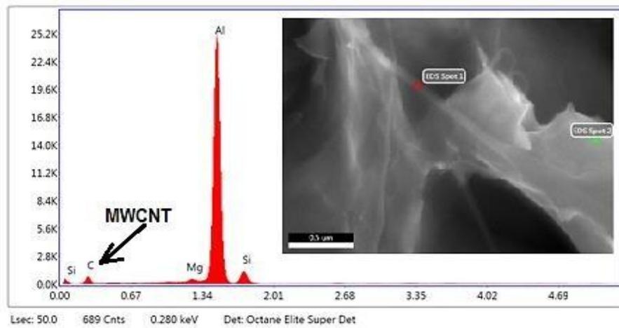
Figure 4.6: FESEM EDX Analysis shows elements in A319 – MWCNT Composite Alloy
