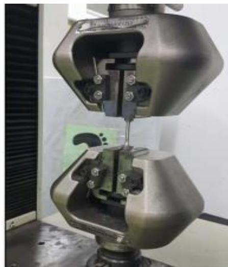
Figure 3.16: Tensile Test Sample
