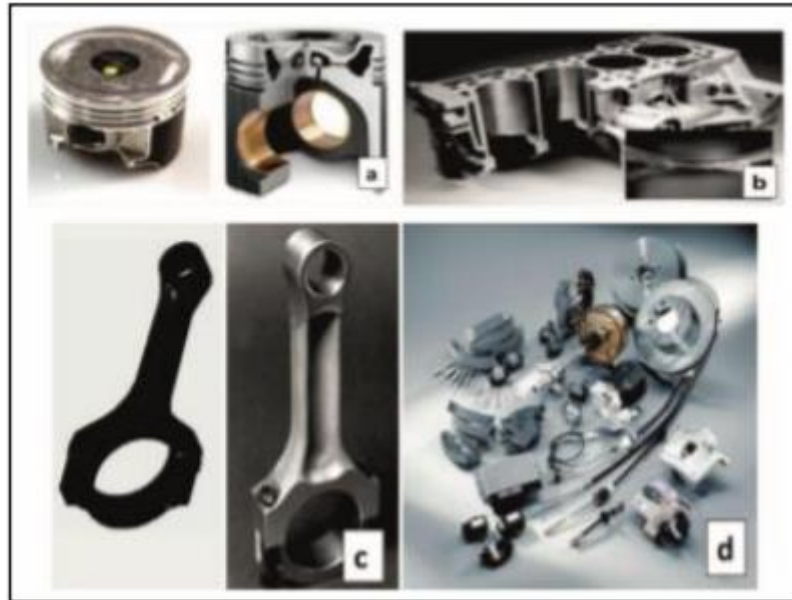
Figure 2.1: Application of metal matrix composites (MMC) (a) piston, (b) engine with cylinder barrel, (c) piston connecting rod, (d) brake 3system (Verma & Khvan, 2019)
