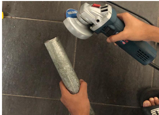
Figure 4.8: Worker performing a manual bevelling process while Hand Arm Vibration Meter detect the vibration produce by the hand grinder.
