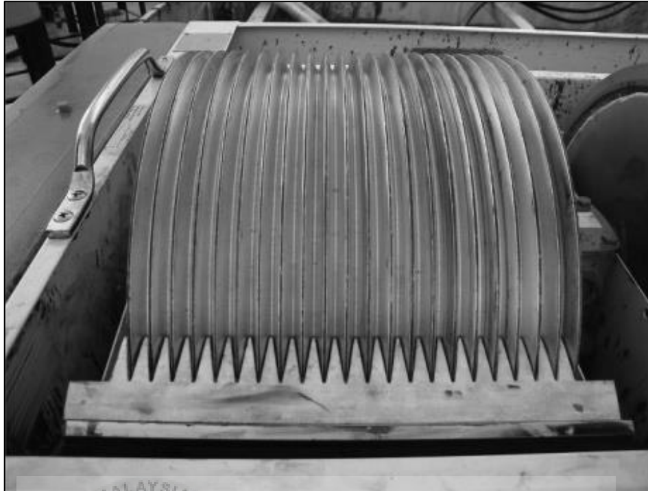
Figure 2.7: Drum with triangular-shaped grooves and matching scraper (Broje and Keller, 2006)
