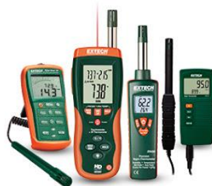
Figure 2.10: Electronic hygrometer (Source: extech.com)
