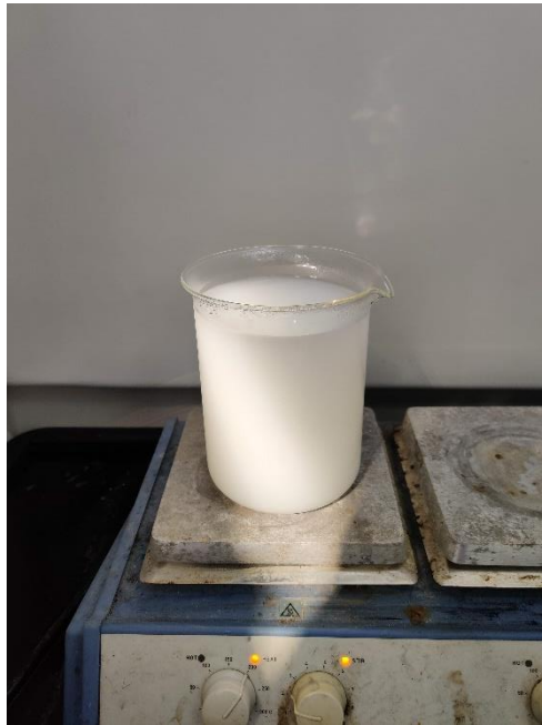
Figure 3.2: Beaker filled with \text{TiOSO}_4 powder was on a hot plate
