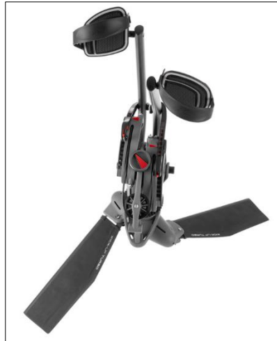
Figure 2.6.1-2: Fin Drive System
