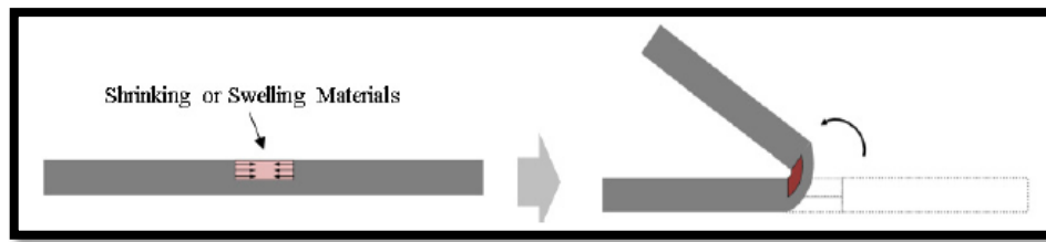
Figure 2.25: Swelling of the layer (Koh et al., 2014).
