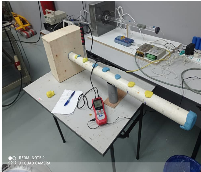
Figure 3.6: The experimental set-up for the test rig of the thermoacoustic system.
