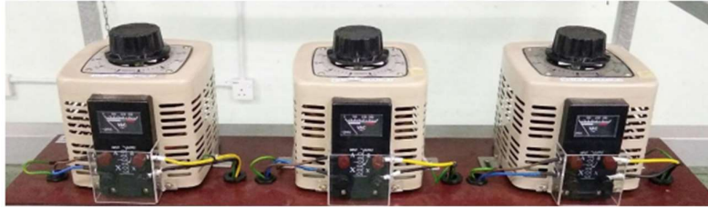
Figure 3.3: Voltage regulator used in ASEL's solar simulator
