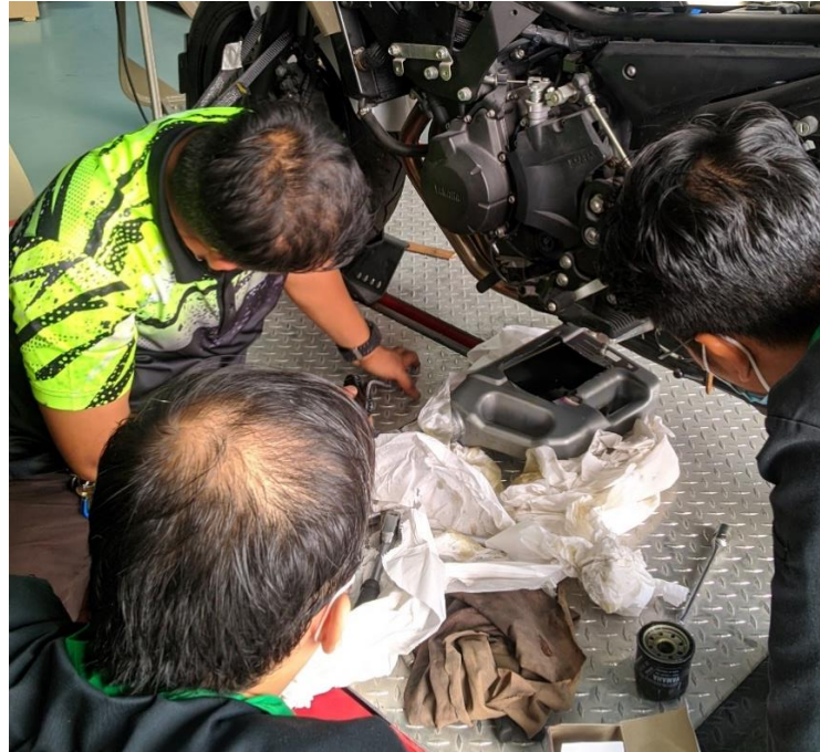
Figure 3.13: Opening the oil port and let used engine oil flow out.
