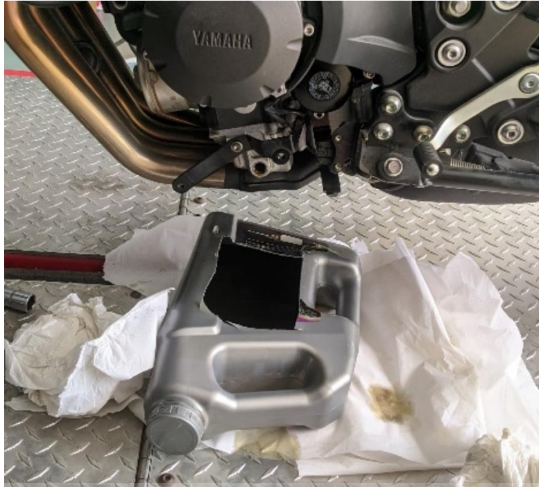
Figure 3.15: Waiting as many used engine oil to flow out as possible
