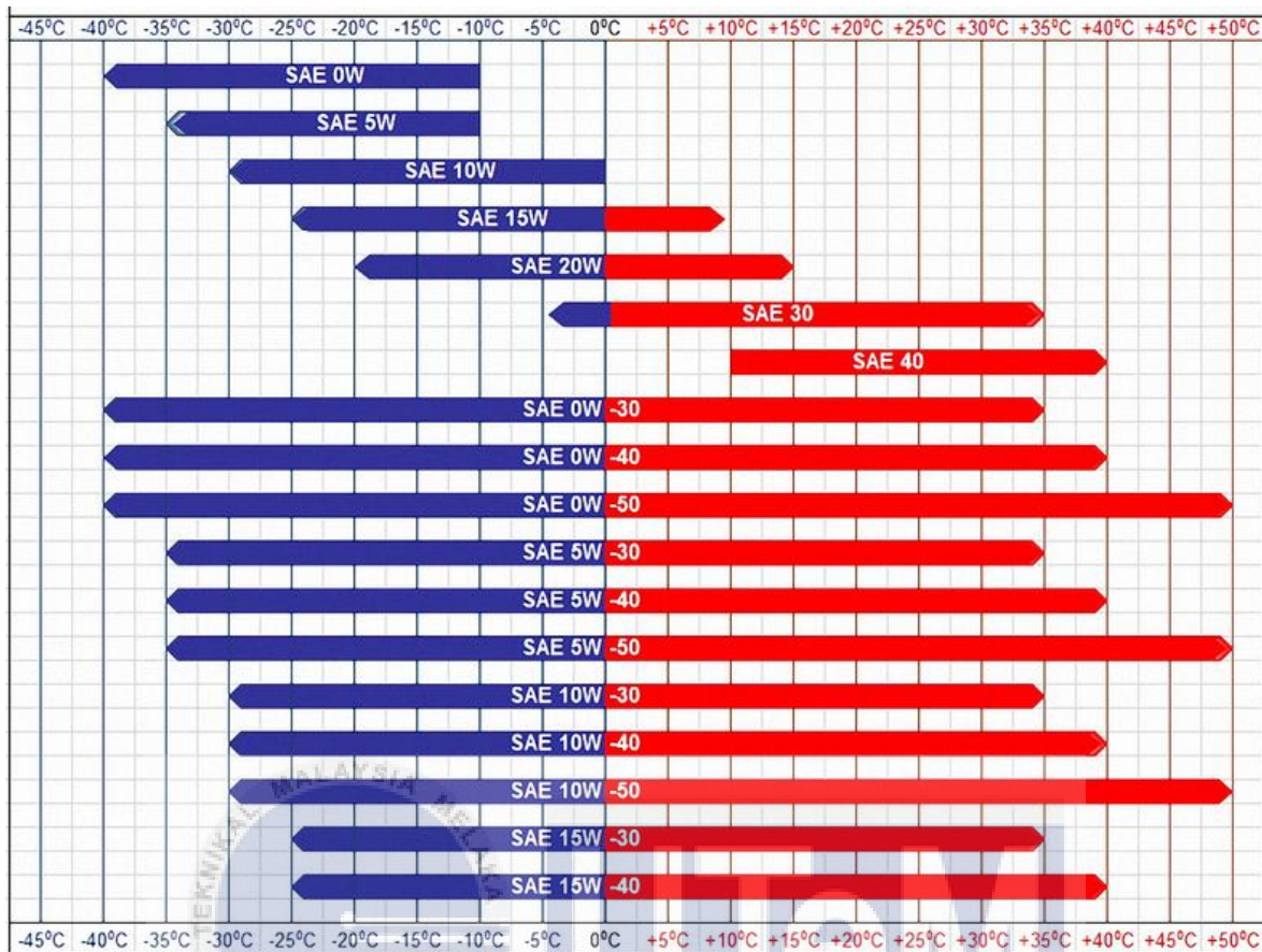
Figure 2.6: Viscosity Chart (Internet Source, Retrieved 10 January 2021).
