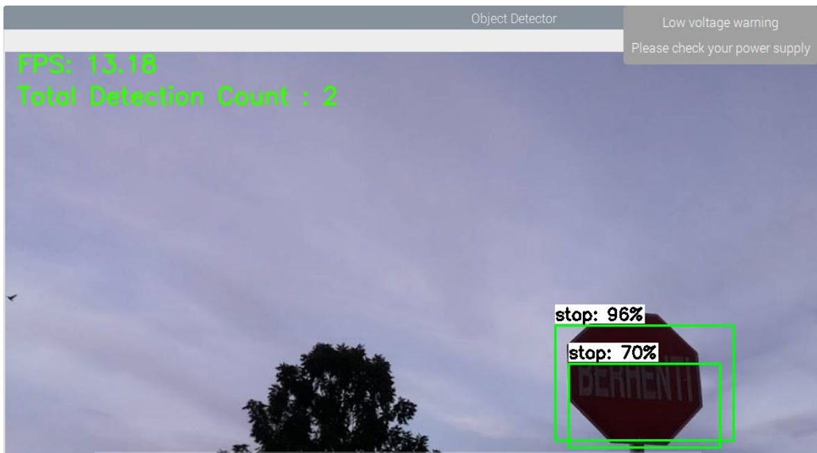
Figure 4.27: ‘Stop’ warning traffic sign is recognised with the highest 96 percent of accuracy
