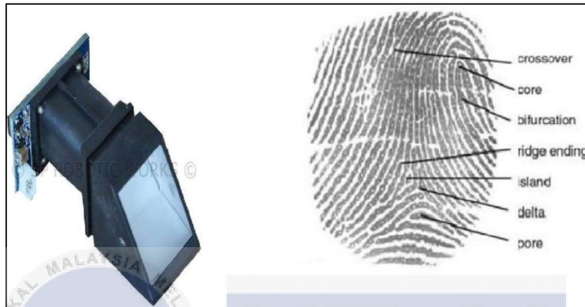
Figure 4(a): R305 Fingerprint module (Sumit Singh, 2015)
