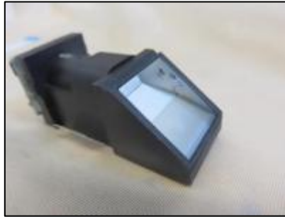
Figure 5(a): Tooan OP-100N optical fingerprint sensor (Kamaraju and Kumar, 2015)
