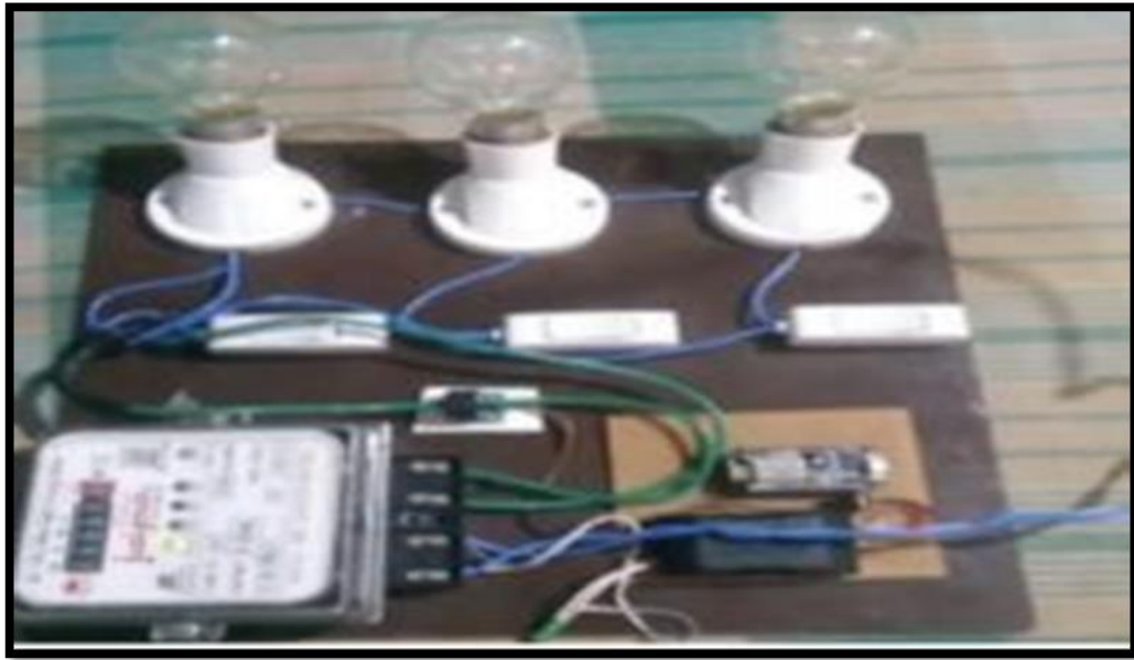
Figure 2.20: The hardware setup for power measurement (Ananth, D.V.N et al., 2019)
