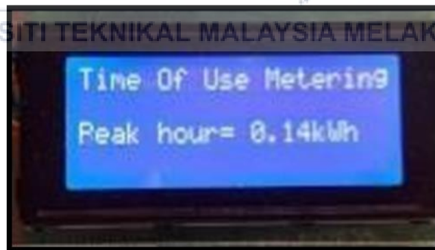
Figure 2.19: The proposed SEM displays ToU (Ali, R.A et al., 2018)
