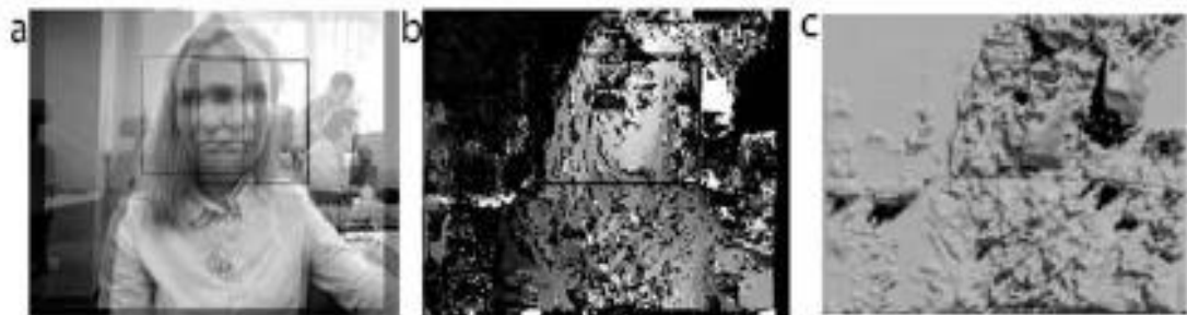
Figure 2.1: (a) combined images; (b) depth map; (c) 3D model of the depth map.
