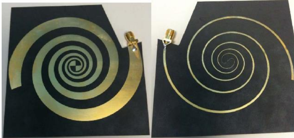
Figure 2.1: Top and bottom view of log spiral antenna
