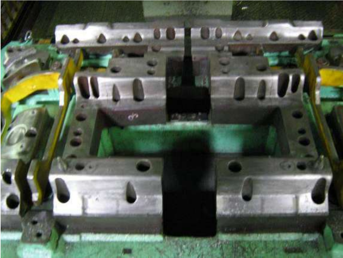
Figure 2.2: Progressive (punch and blanking) die with strip and punching.
