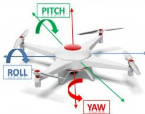
Figure 2.4: Roll, Pitch, and Yaw moment
