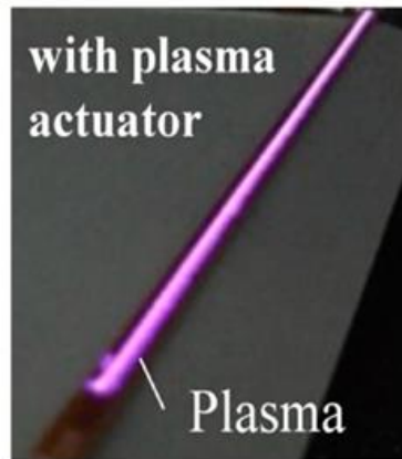
Figure 2.2 Ionized air over electrode covered by dielectric layer
