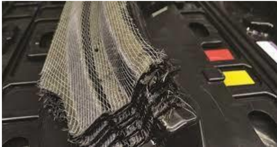
Figure 2.1 Outcomes from conventional method of trimming CFRP
