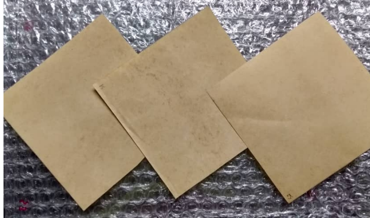
Figure 2.2: The thermally upgraded kraft paper used for testing.
