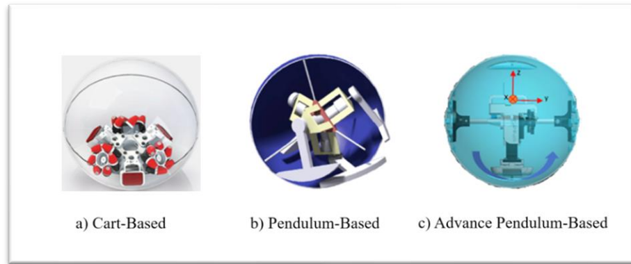
Figure 2.1 Centre of Mass Manipulation drive mechanisms
