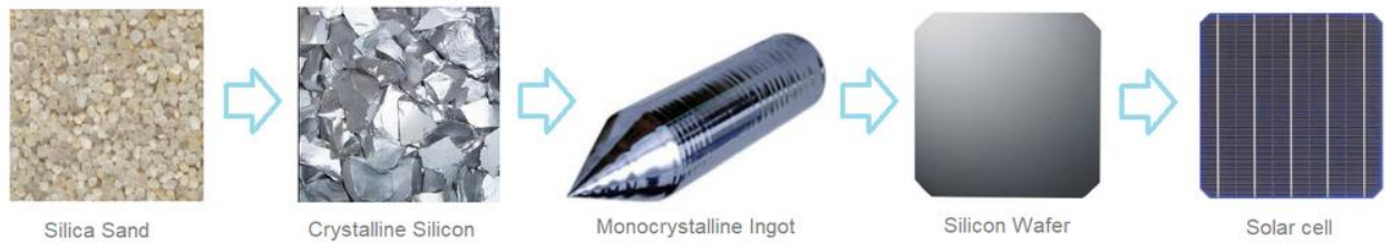
Figure 2-2 Solar Cell Manufacturing Process [5]
