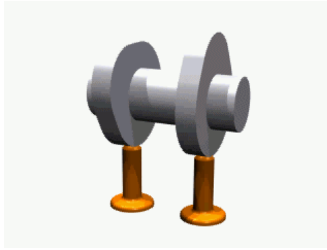
Figure 2.4 Constantly spinning cams that produce the supporters of the cam's rotating linear motion
