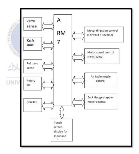
Figure 1.1: Paper cutting machine using ARM7 system
