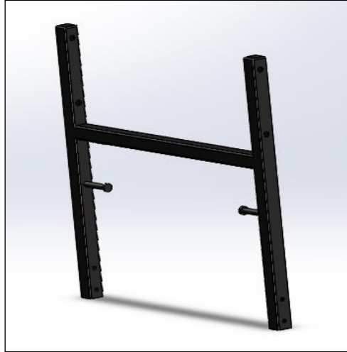
Figure 3.14: Square Hollow Bar H Shape
