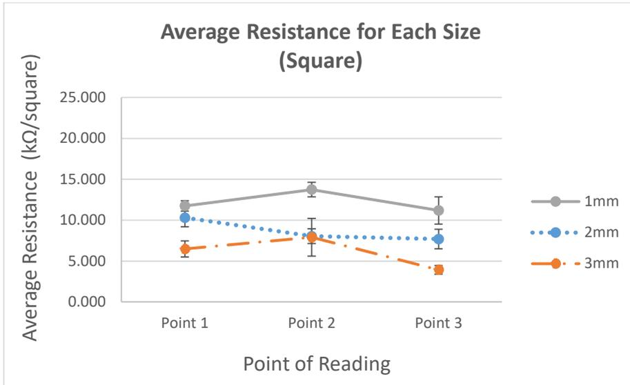
Figure 4. 11: Graph of Average Resistance between Sizes, 1mm, 2mm and 3mm for Temperature 110 °C for Square Pattern
