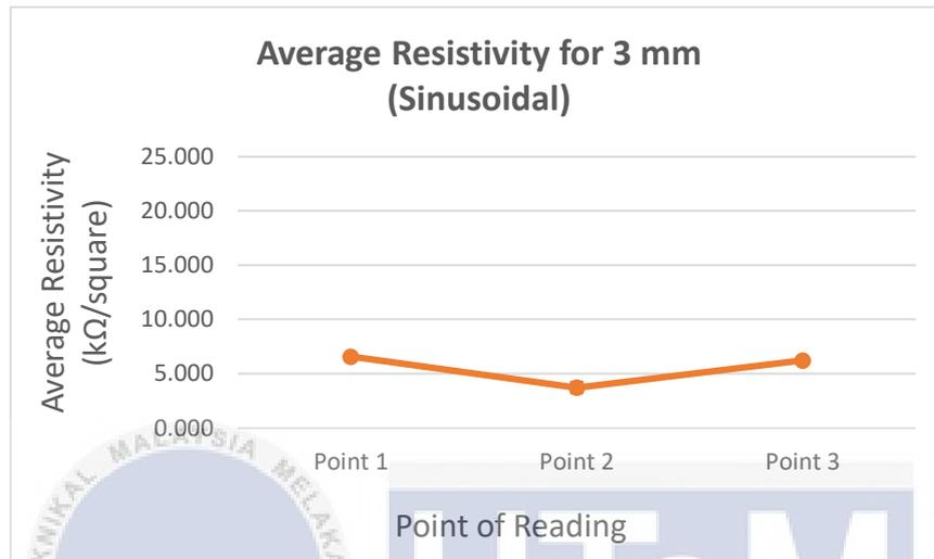
Figure 4. 47: Graph of Average Resistivity for Sample 2 Width 3 mm Pattern Sinusoidal
