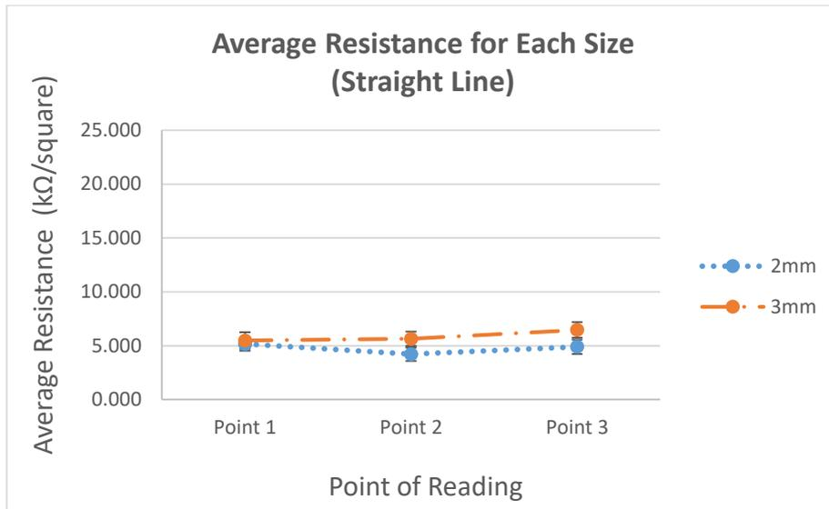
Figure 4. 9: Graph of Average Resistance between Sizes, 2mm and 3mm for Temperature 110 °C, Pattern Straight Line
