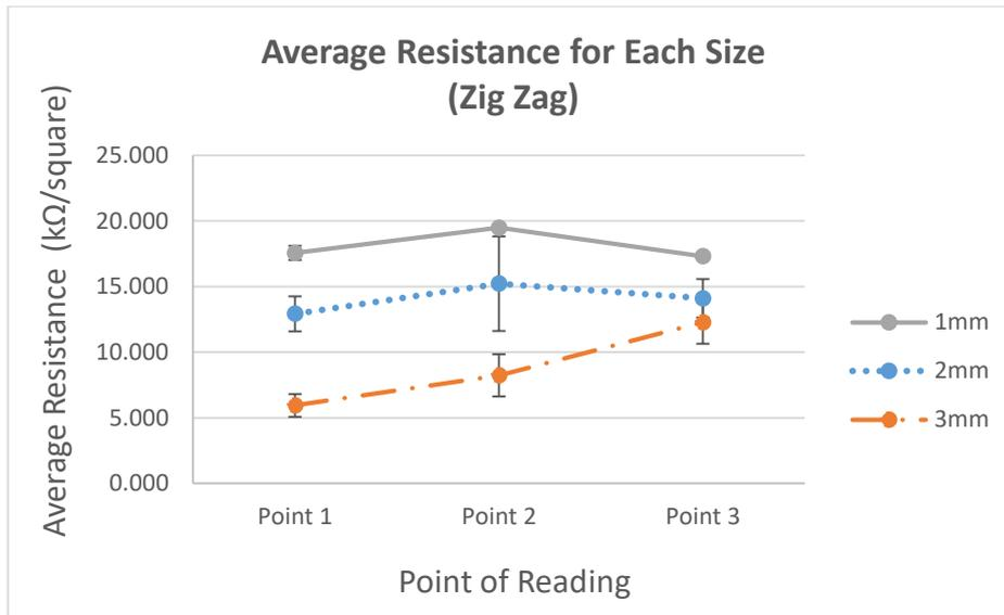
Figure 4. 10: Graph of Average Resistance between Sizes, 1mm, 2mm and 3mm for Temperature 110 °C, Pattern Zig Zag
