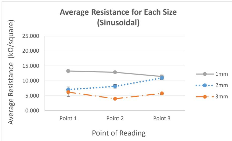
Figure 4. 12: Graph of Average Resistance between Sizes, 1mm, 2mm and 3mm for Temperature 110 °C, Pattern Sinusoidal
