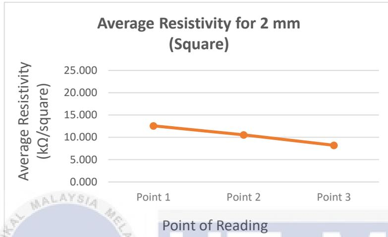
Figure 4. 36: Graph of Average Resistivity for Sample 2 Width 2 mm Pattern Square
