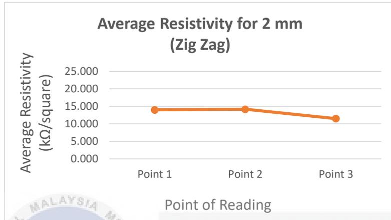
Figure 4. 42: Graph of Average Resistivity for Sample 2 Width 2 mm Pattern Zig Zag
