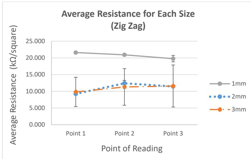
Figure 4. 2: Graph of Average Resistance between Sizes, 1mm, 2mm and 3mm for Temperature 90 °C Pattern Zig Zag
