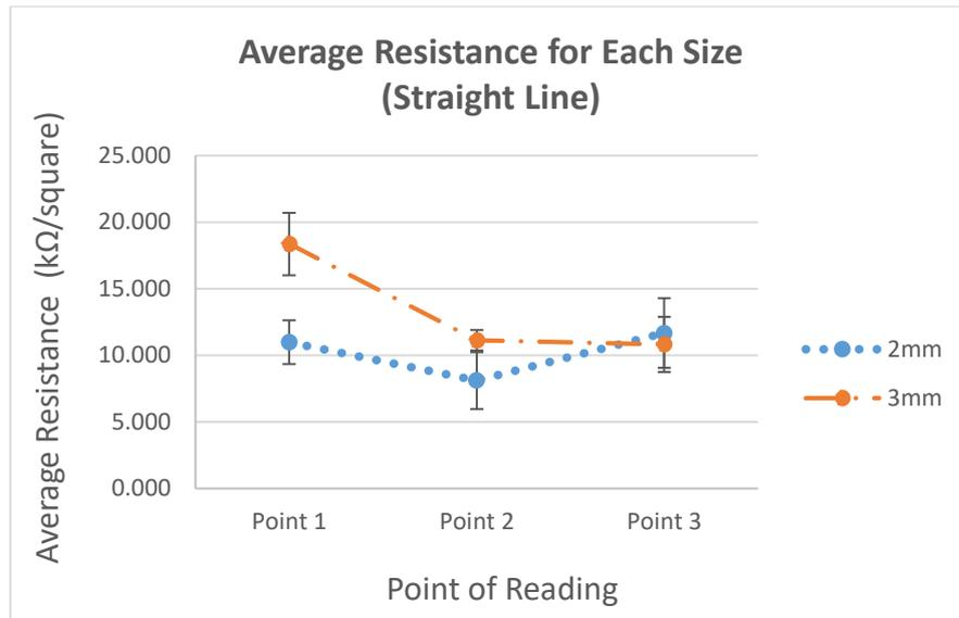
Figure 4. 1: Graph of Average Sheet Resistance between Sizes, 2mm and 3mm for Temperature 90 °C Pattern Straight Line
