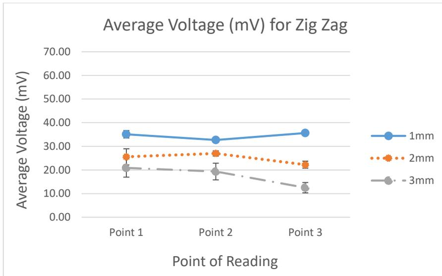
Figure 4. 22: Graph of Average Voltage between Sizes, 1mm, 2mm and 3mm for Temperature 110 °C for Zig Zag Pattern
