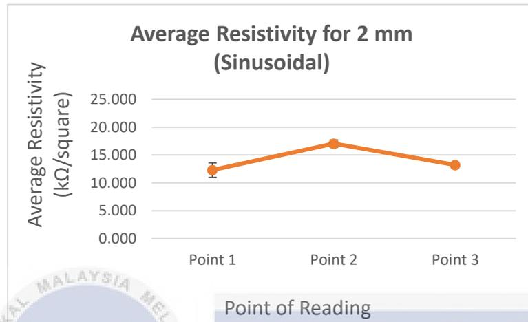
Figure 4. 31: Graph of Average Resistivity for Sample 2 Width 2 mm Pattern Sinusoidal
