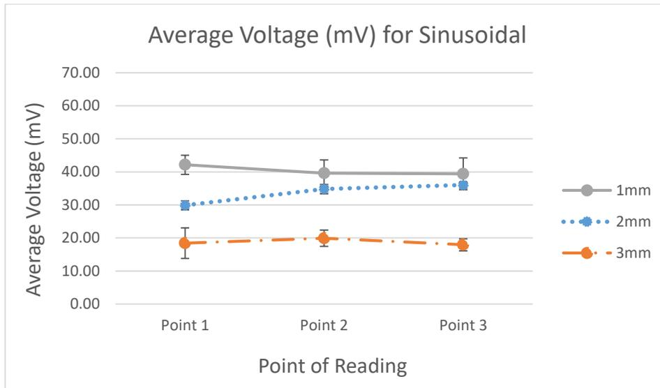
Figure 4. 16: Graph of Average Voltage between Sizes, 1mm, 2mm and 3mm for Temperature 90 °C for Pattern Sinusoidal
