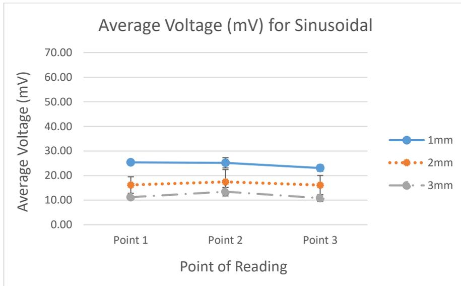
Figure 4. 24: Graph of Average Voltage between Sizes, 1mm, 2mm and 3mm for Temperature 110 °C for Sinusoidal Pattern
