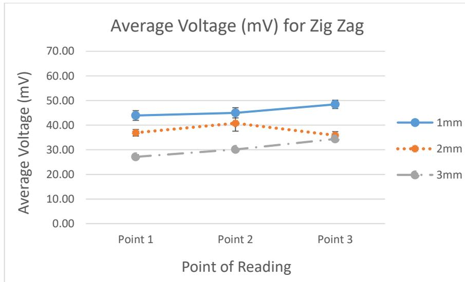
Figure 4. 18: Graph of Average Voltage between Sizes, 1mm, 2mm and 3mm for Temperature 100 °C for Pattern Zig Zag
