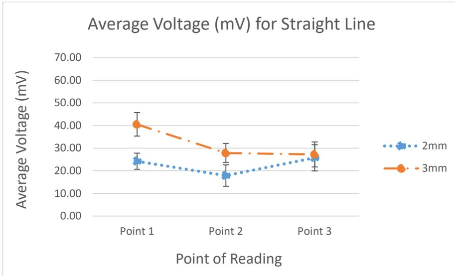
Figure 4. 13: Graph of Average Voltage between Sizes, 2mm and 3mm for Temperature 90 °C for Pattern Straight Line
