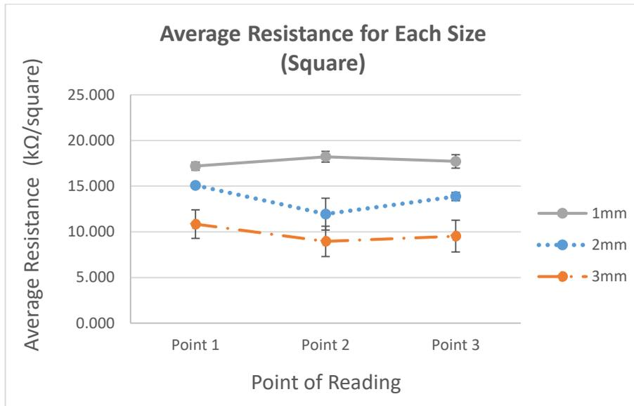
Figure 4. 3: Graph of Average Resistance between Sizes, 1mm, 2mm and 3mm for Temperature 90 °C Pattern Square
