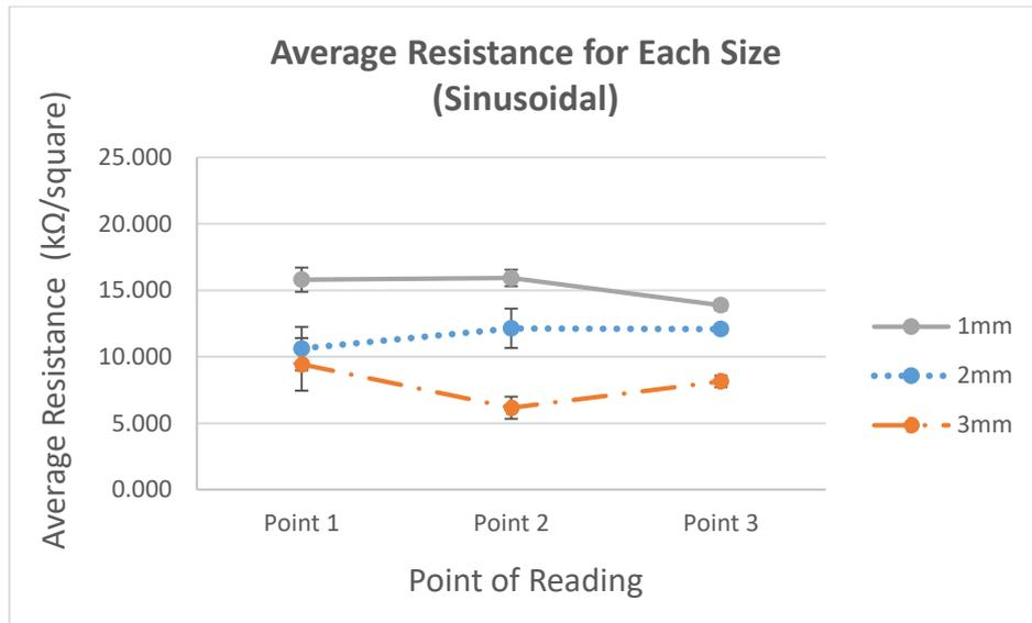
Figure 4. 8: Graph of Average Resistance between Sizes, 1mm, 2mm and 3mm for Temperature 100 °C, Pattern Sinusoidal
