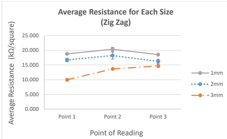
Figure 4. 6: Graph of Average Resistance between Sizes, 1mm, 2mm and 3mm for Temperature 100 °C Pattern Zig Zag
