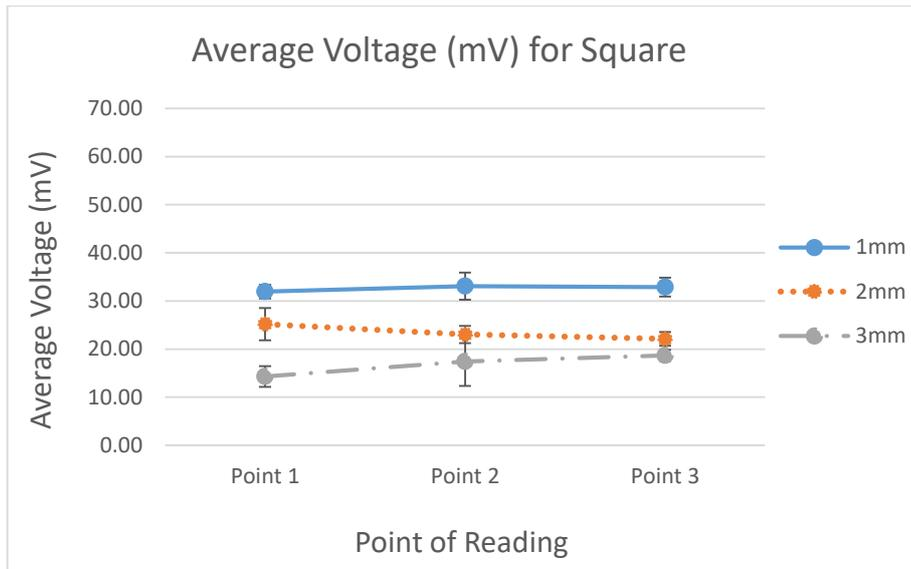
Figure 4. 19: Graph of Average Voltage between Sizes, 1mm, 2mm and 3mm for Temperature 100 °C for Square Pattern
