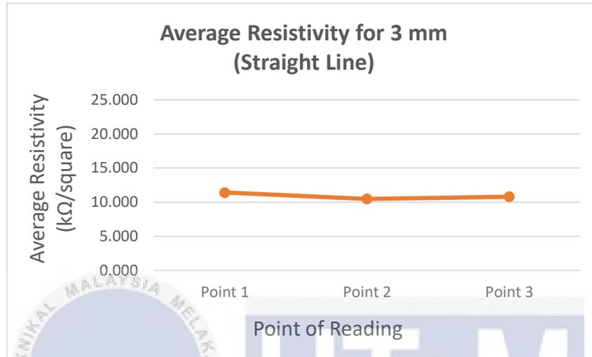
Figure 4. 33: Graph of Average Resistivity for Sample 2 Width 3 mm Pattern Straight Line
