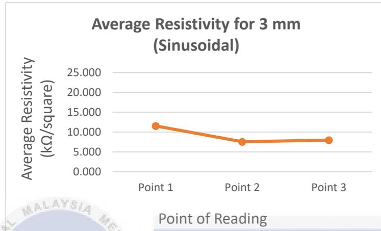
Figure 4. 39: Graph of Average Resistivity for Sample 2 Width 3 mm Pattern Sinusoidal
