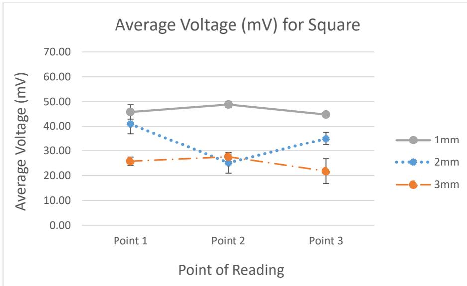
Figure 4. 15: Graph of Average Voltage between Sizes, 1mm, 2mm and 3mm for Temperature 90 °C for Pattern Square
