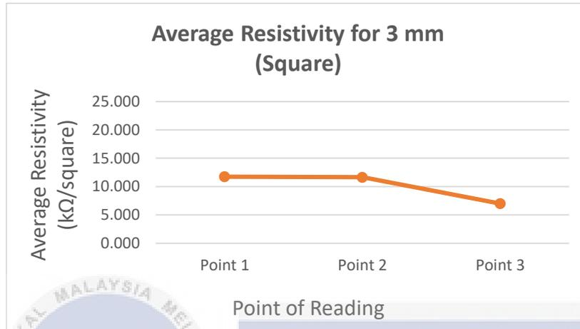
Figure 4. 30: Graph of Average Resistivity for Sample 2 Width 3 mm Pattern Square
