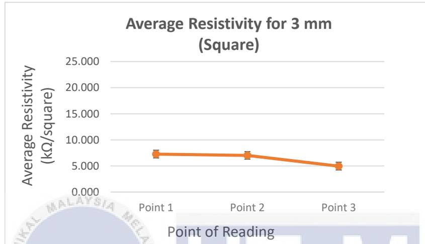
Figure 4. 45: Graph of Average Resistivity for Sample 2 Width 3 mm Pattern Square
