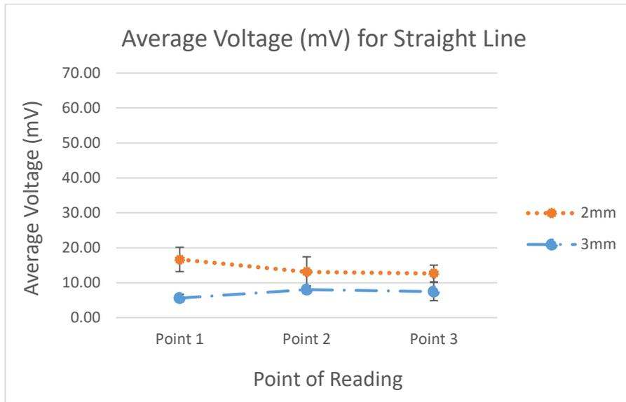
Figure 4. 21: Graph of Average Voltage between Sizes, 2mm and 3mm for Temperature
