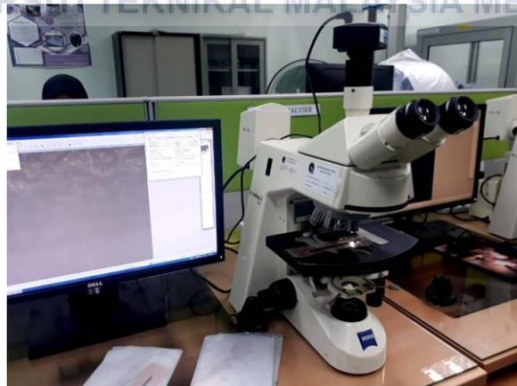
Figure 3. 9: Light Microscope
