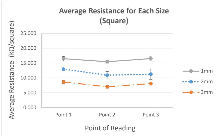
Figure 4. 7: Graph of Average Resistance between Sizes, 1mm, 2mm and 3mm for Temperature 100 °C Pattern Square
