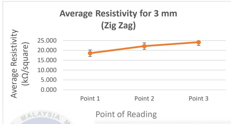
Figure 4. 28: Graph of Average Resistivity for Sample 2 Width 3 mm Pattern Zig Zag
