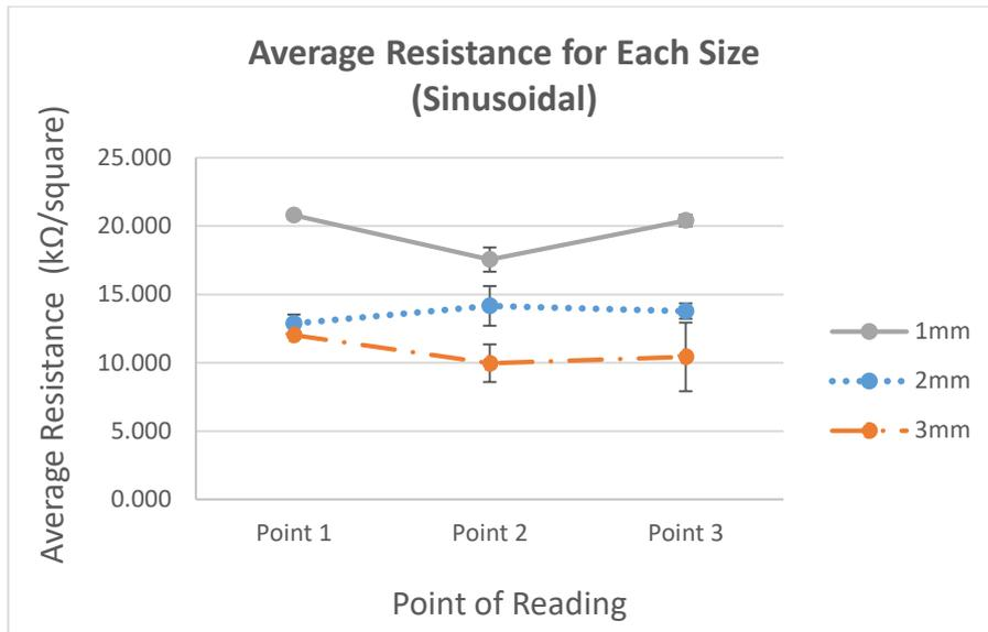
Figure 4. 4: Graph of Average Resistance between Sizes, 1mm, 2mm and 3mm for Temperature 90 °C Pattern Sinusoidal
