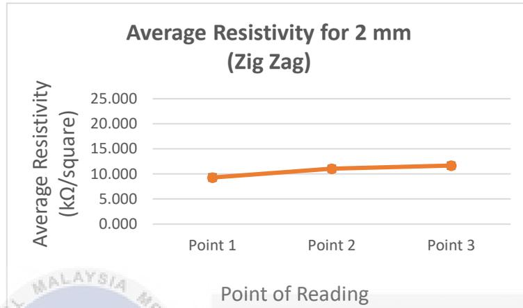
Figure 4. 27: Graph of Average Resistivity for Sample 2 Width 2 mm Pattern Zig Zag
