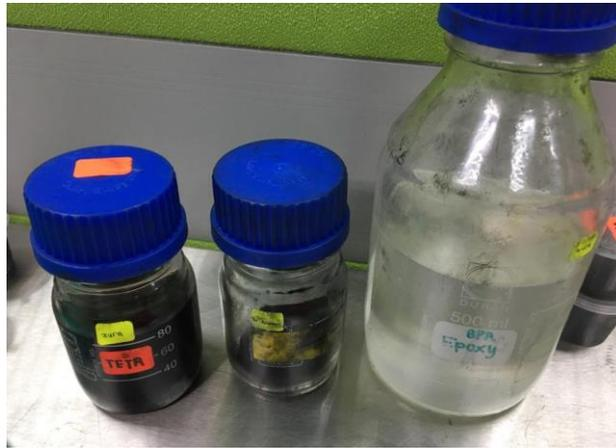
Figure 3. 2: Material Used for Process of Composition; Hardener, Graphene Nanoplatelets, Epoxy
