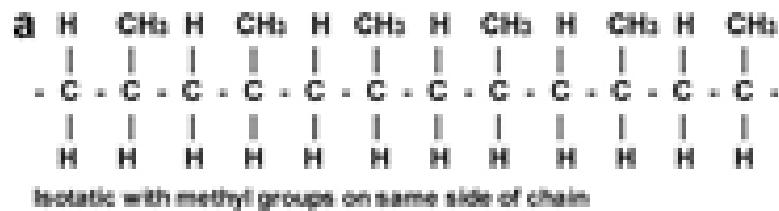
Figure 2.2 Schematic of polypropylene tacticities isotactic with all methyl groups on the same side of the chain
