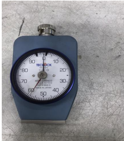
Figure 3.22 Analog scale "D" type Durometer
