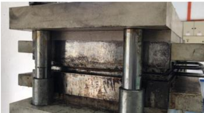
Figure3.17 Hot pressing process carried out
