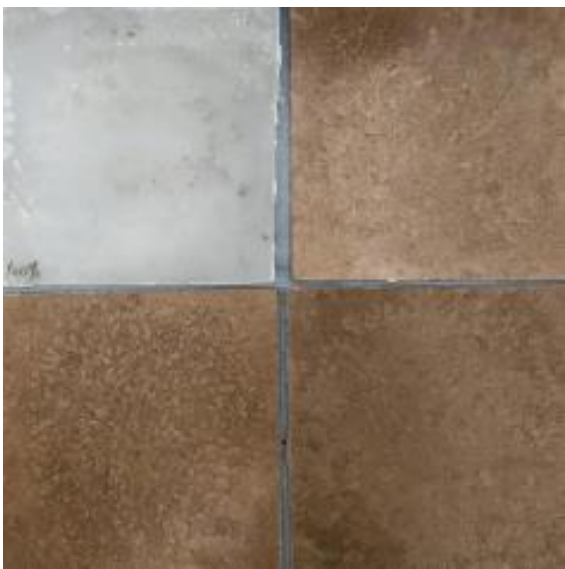
Figure 3.18 pressed samples (100%, 20%,30%,40% php-pp)
