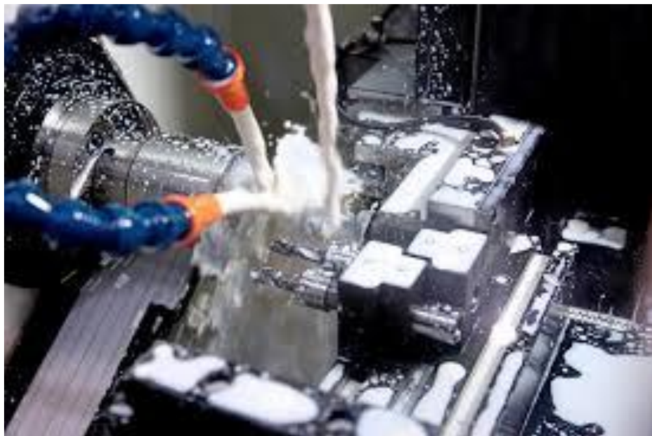
Figure 1.2: Coolant system in CNC turning (Source: https://www.sundry.com/whats-different-between-cnc-turning-and-cnc-milling/ )
