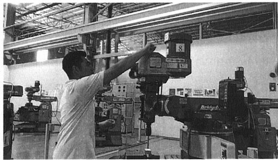
Figure 1.6: The drawbar is at overhead height
