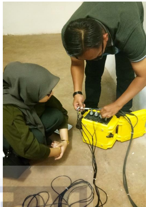
Connecting various sensor probe into data powerlogger
