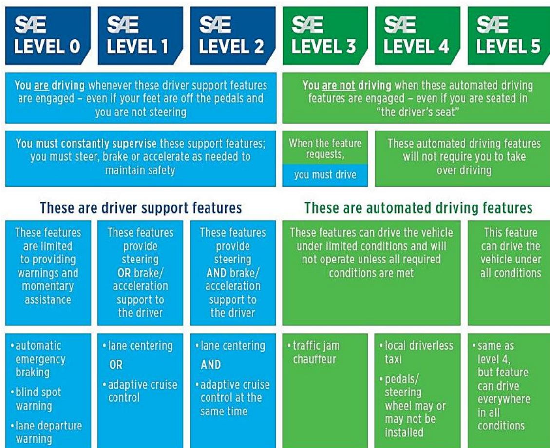
Figure 2.2: Level of automation based on SAE (Source: Jennifer, 2019)
