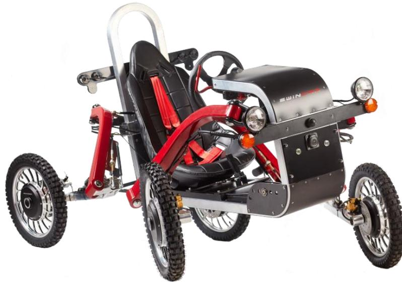
Figure 1.3: Example of pendular vehicle
