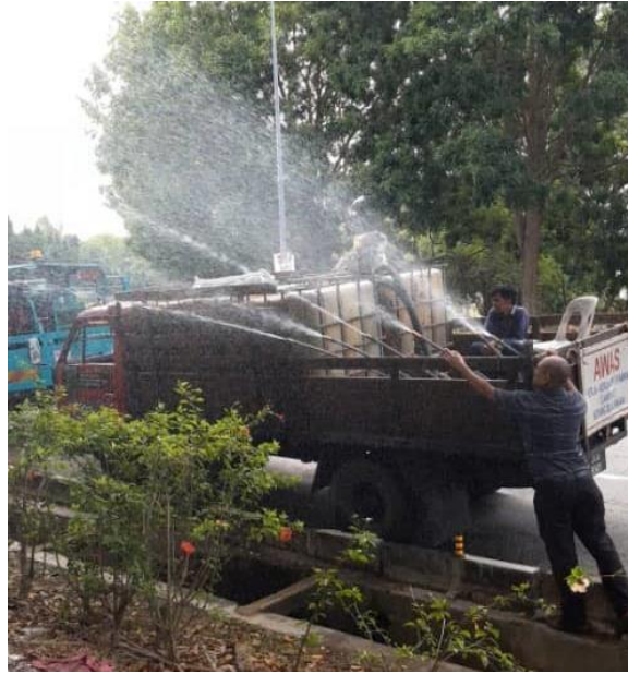
Figure 3.30: Connected rain simulator at the lorry
