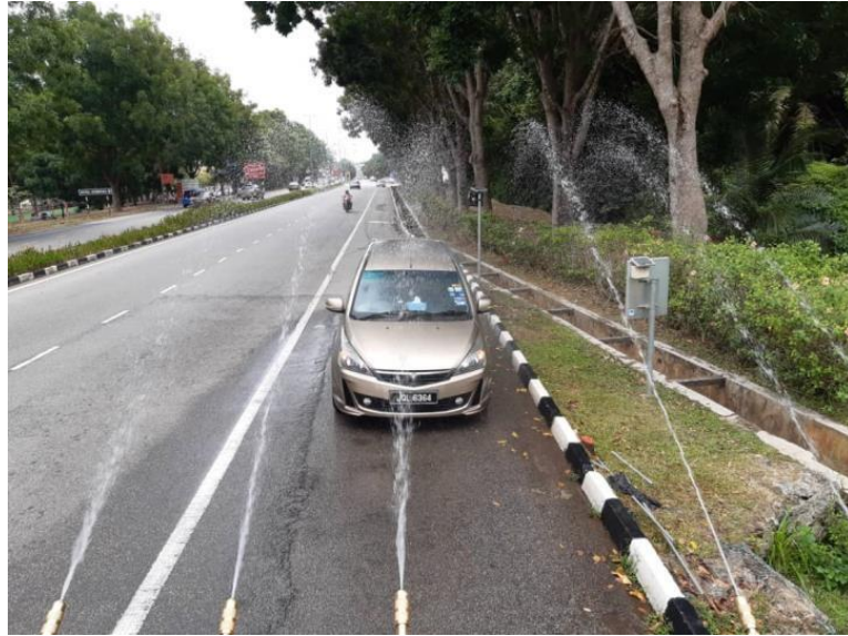
Figure 3.31: Rain simulator spurting out water towards static car
