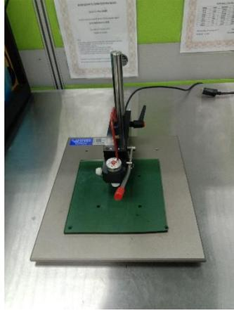
**Figure 3.11:** A JANDEL Four-Point Probe Test.
