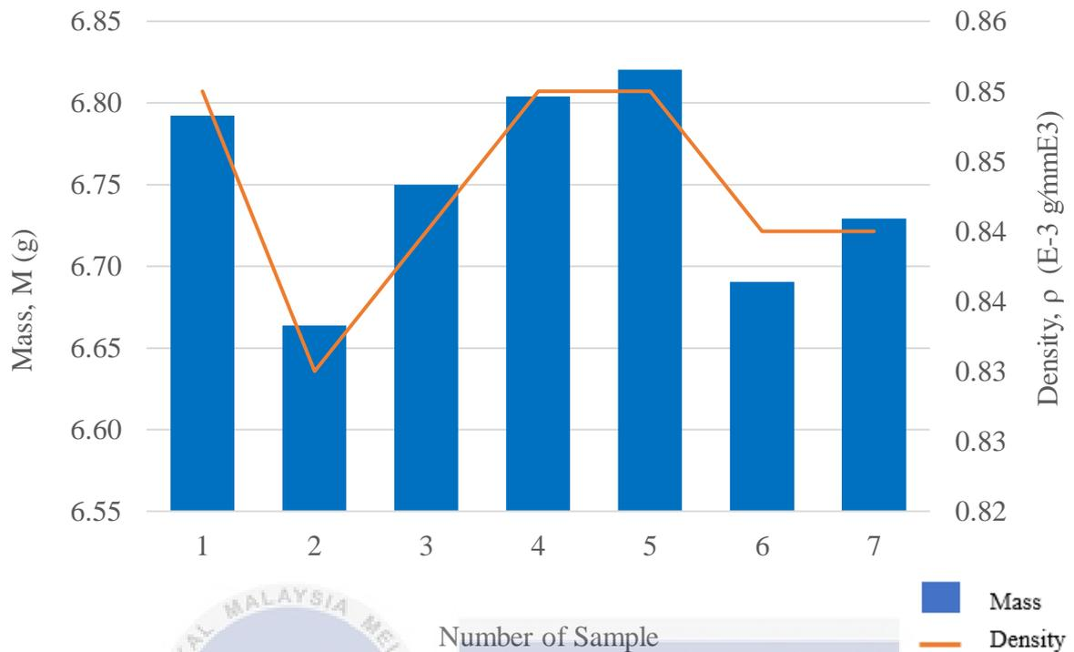
**Figure 4.8:** Graph of mass and density for GNP/UHMWPE-0.3 composite sample.
