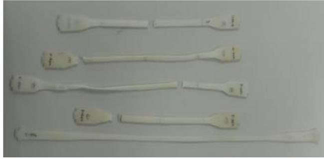
**Figure 4.21:** Neat UHMWPE sample after tensile test.
