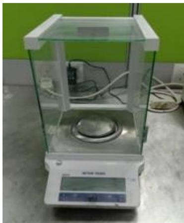
**Figure 3.3:** Electronic balance.
