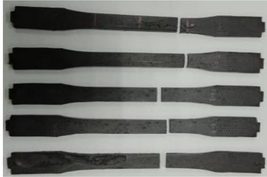
**Figure 4.29:** GNP/UHMWPE-1.0 composite samples after tensile test.
