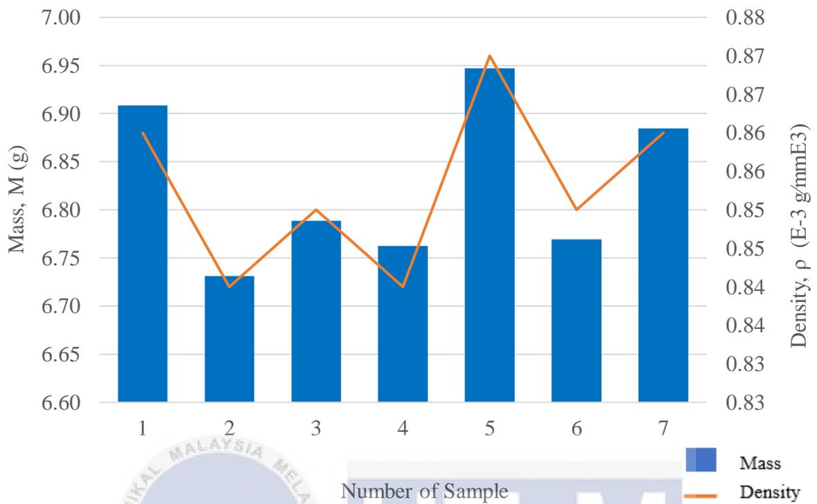
**Figure 4.10:** Graph of mass and density for GNP/UHMWPE-1.0 composite sample.
