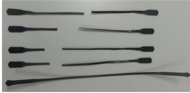
**Figure 4.25:** GNP/UHMWPE-0.3 composite samples after tensile test.
