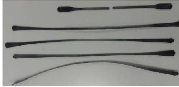
**Figure 4.23:** GNP/UHMWPE-0.1 composite samples after tensile test.
